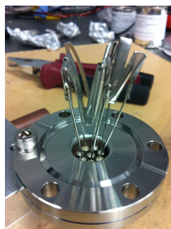
Fig. 2.3 Atom sources spot welded to the UHV electrical feedthrough
