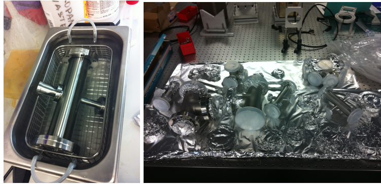
Fig. 2.4 On the left: the vacuum system part immersed in an acetone ultrasonic bath. On the right: the parts, wrapped in aluminum foil, laid down on the table after cleaning.
